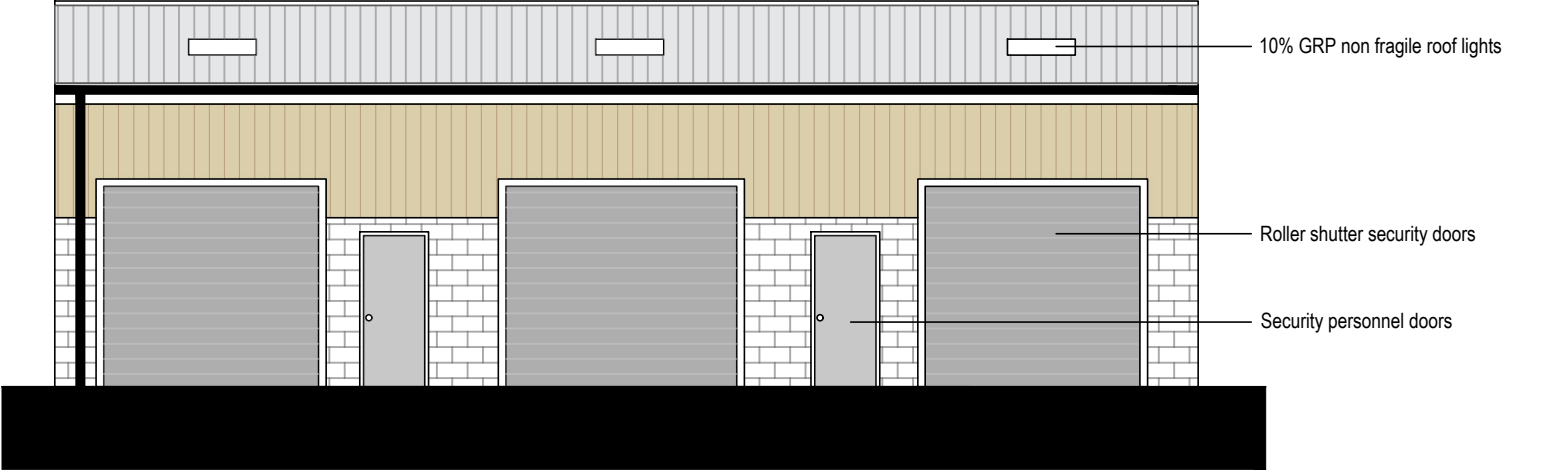
Front Elevation (West)
