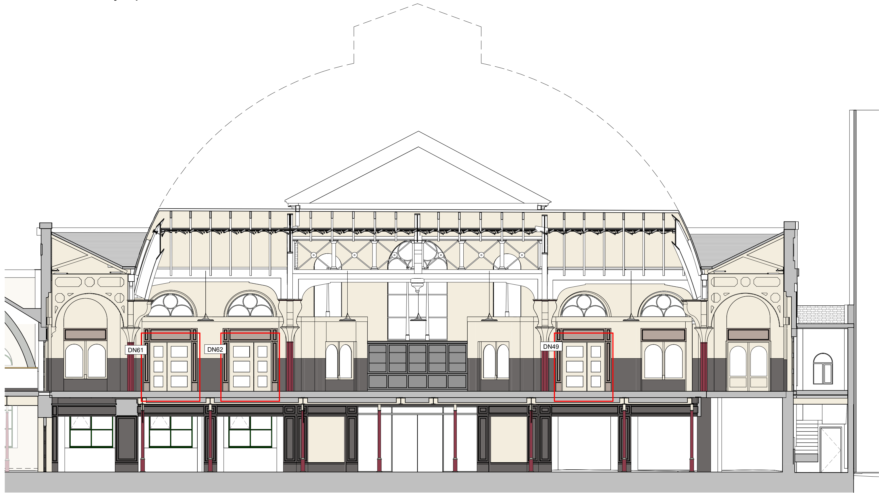
1 Proposed Door Accessibility Improvements - East Elevation 1 : 100
